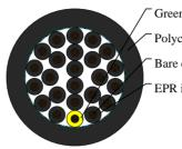
Green/Yellow wire Polychloroprene rubber outer jacket Bare copper conductor EPR insulation
